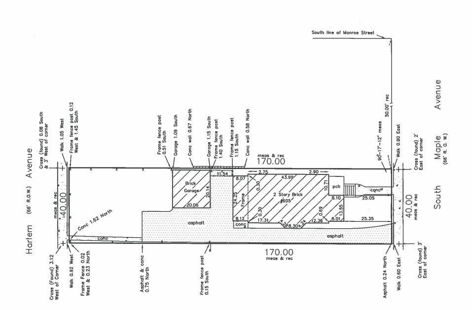
LEGEND meas = measured, E = East rec = record, S = South R.O.W. = right-of-way conc = concrete, W = West
