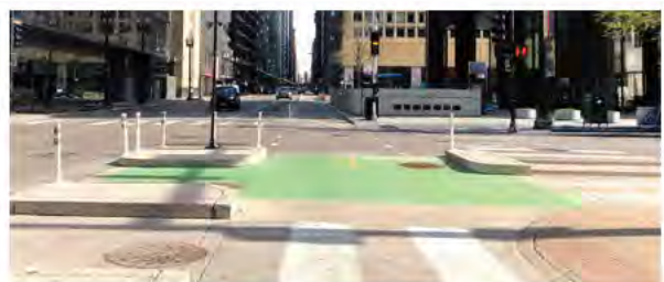
Example of a protected intersection.
